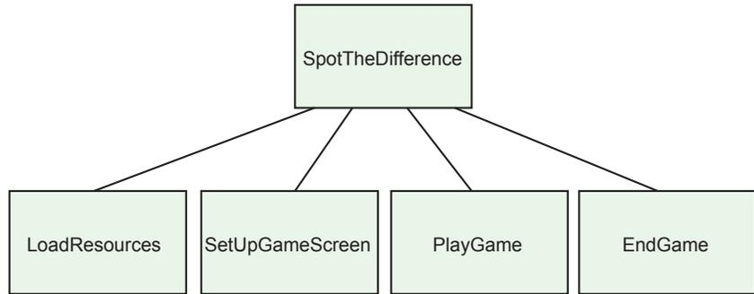
Finally, we add any parameters passed between the routines. In this case *PlayGame* returns the time taken to find all the differences and *EndGame* takes that same value as an *In* parameter. Parameters are represented by labelled, directed circles (see FIG-8.13).
